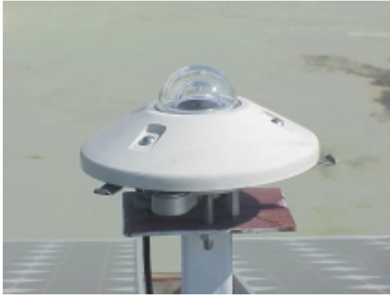
Figure 10.4: Kipp & Zonan CM11 Pyranometer.
