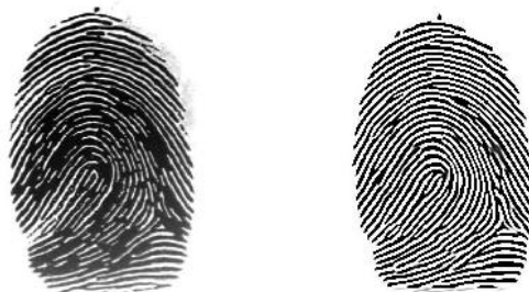
Figure 3. An input image and the corresponding image after enhancement
