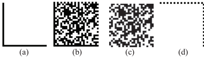
Figure 1. Data matrix barcode structure example: (a),(d) Finder pattern (b) Whole barcode, and (c) Data cell
