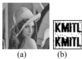
Fig. 6: Result of Low-pass filtering (a) Watermarked image (b) Extracted watermark.
